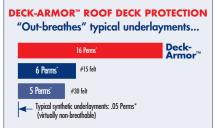
\*Nominal MVTR perms value as measured by GAF on Mocon unit @ 82°F (28°C) and 50% R.H.
